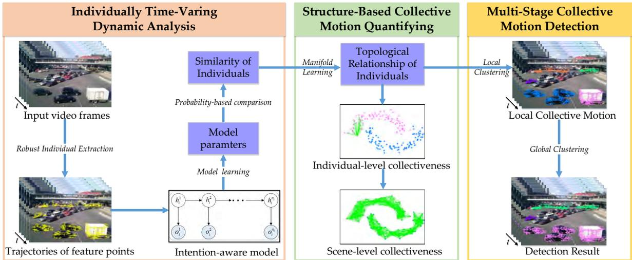
Fig. 2. The pipeline of the proposed framework. First, we extract motions of individuals with robustness, and propose an intention-aware model to analyze time-varying motion dynamics. Then a collectiveness measurement, which investigates the topological relationship between individuals, is utilized to measure collectiveness. Finally, a multi-stage clustering strategy is developed to detect collective motions in crowd scenes.
