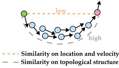
Fig. 4. Illustration of topological relationship. The red and green point show low similarity on spatial location and moving direction, but they are consistent from the topologic perspective. Best viewed in color.
